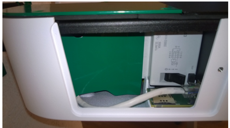
Fig. 7 G7 station with installed RCD protection unit
